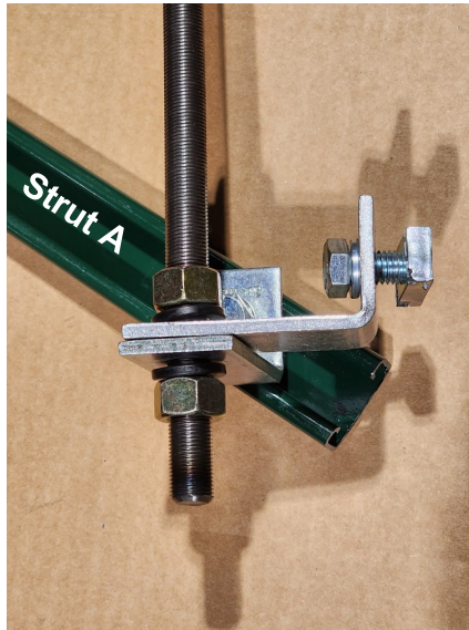
Figure 10 Strut "A" "lower end" Strut, Bracket & Channel Nut Assembly "Overlapping, Right Angle" Brackets
