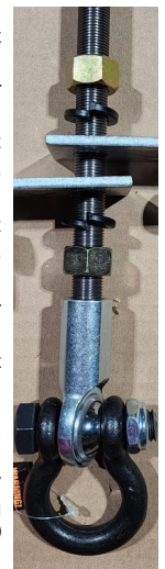
Figure 8 Threaded Rod Bottom End Hardware Attachment Order Detail:
