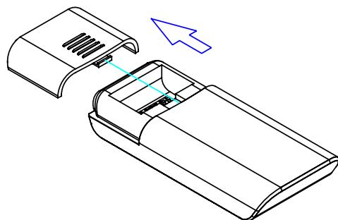
4. Make sure the Setting of the DIP SWITCH is the same as the PIN code sticker.
