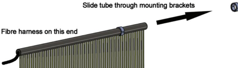
Secure the wall tube to the brackets by tightening the supplied grub screws into the top holes on the brackets.
